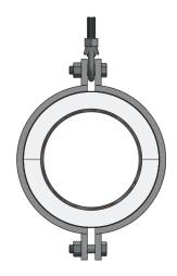
Pre-Insulated Pipe Supports possess a beneficial energy saving feature over conventional pipe supports. They are designed to keep energy where it belongs, in the pipe. The weight of the mechanical system is supported by high compressive strength, load bearing insulation. This thermally isolates the pipe from the surrounding environment by allowing the insulation system and its vapor barrier to pass continuously through the pipe support.
