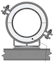
Load Bearing Insulation Prevents Heat Flow
